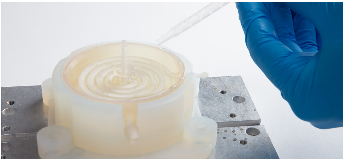
Adhesive being applied to a part in a bonding jig printed in Formlabs Durable Resin.
