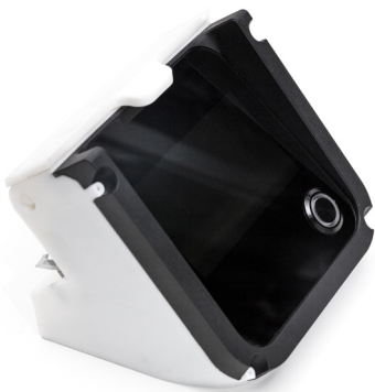
An assembly jig used for manufacturing the Formlabs Form 2 3D printer.
