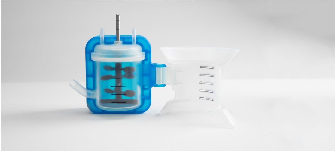
Hinged jig for applying volumetric markings, printed with Formlabs Tough Resin and Durable Resin.
